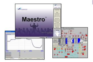
The Maestro™ Control System is designed to meet the most demanding lyophilization requirements of pharmaceutical and biotechnology companies. The system utilizes the GE Fanuc Proficy® HMI/SCADA – iFIX solution for Windows and an Allen-Bradley 5/03 or 5/05 Small Programmable Logic Controller (SLC). The software system meets all Current Good Manufacturing Practice (cGMP) standards and regulatory guidelines for computer systems used for pharmaceutical processing equipment and is fully validateable.
